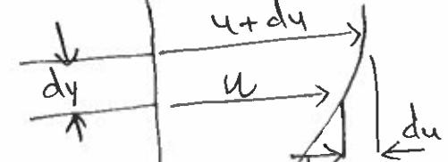
say  $u + du$  as shown in fig. The viscosity together with relative velocity causes a shear stress acting b/w the fluid layers.
