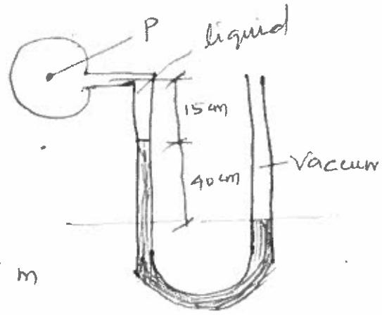
height of liquid  $h_1 = 15 \text{ cm} = 0.15 \text{ m}$
