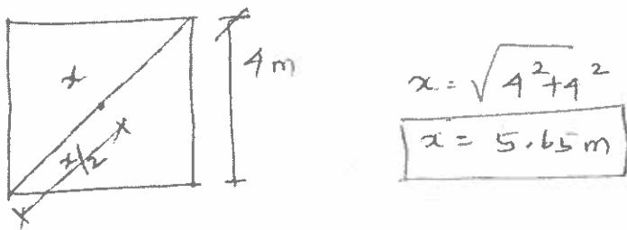
Given:- Size of plate  $4\text{m} \times 4\text{m}$
