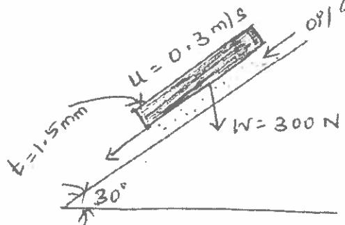
Given :- Size of plate =  $0.8\text{ m} \times 0.8\text{ m}$
