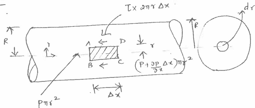
Viscous flow through a pipe
