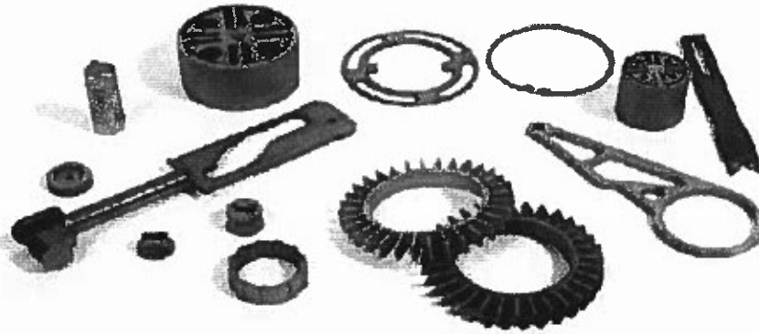
Figure 3: Difficult internal parts made by EDM process working
